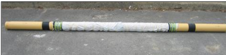
Figure 5. MPSP standpipe with barrier bag.
